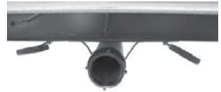
Black/Grey Tank Drain and Valves
